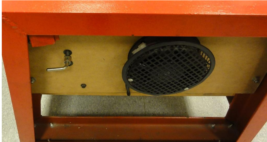
Fig.17. The 12V cut-off switch on the side of the stand
