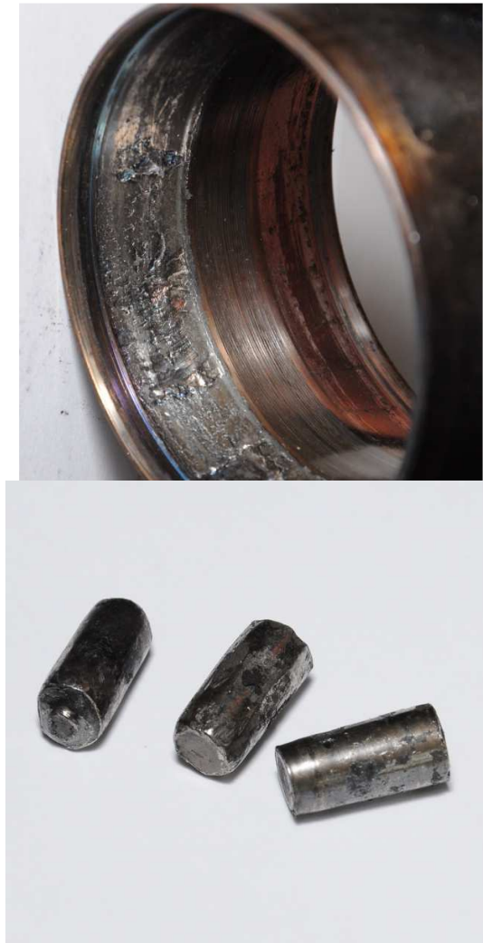
Fig. 1. Worn elements of the wheel bearing.
