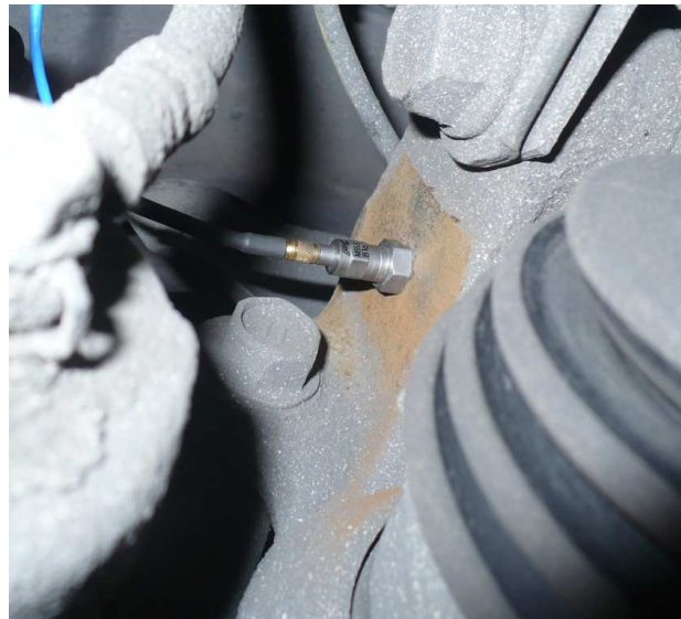
Fig. 5. Placement of mounting of vibration acceleration sensor
