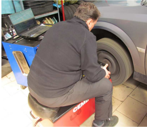
Fig. 4. View of the vehicle together with the dynamic balancing machine used in the research.
