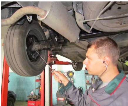
Fig. 2. Testing bearing arrangement of the wheels using stethoscopes, a) classical , b) with amplifier
